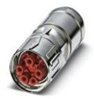
Cable connector, straight long, shielded: yes, SPEEDCON locking, M40, No. of pos.: 8+4+PE, type of contact: Socket, Crimp connection, cable diameter range: 9 mm ... 14 mm
