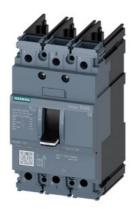
circuit breaker 3VA5 UL frame 125 breaking capacity class S 25kA @ 480V 3-pole, line protection TM210, FTFM, In=20A overload protection Ir=20A fixed short-circuit protection Ii=15 x In UL 489 SB (naval), 50° C without connection
