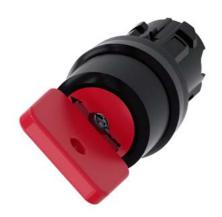
Key-operated switch O.M.R, 22 mm, round, plastic, lock number 73037, red, with 2 keys, 2 switch positions O<I, momentary contact type, Actuating angle 45°, 10:30h/12h, key removal O, with laser labeling, inscription or symbol Customer-specific selection with SIRIUS ACT configurator (CIN)
