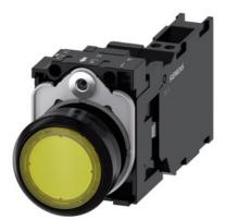
Illuminated pushbutton, 22 mm, round, plastic, yellow, pushbutton, flat, momentary contact type, with holder, 1 NO+1 NC, LED module with integrated LED 24 V AC/DC, spring-type terminal, with laser labeling, symbol number according to, ISO 7000 or IEC 60417
