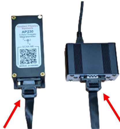
Figure 3 AP230 Connected to Interface Box with the Interface Cable Provided
