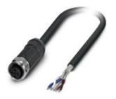
Bus system cable, CANopen<sup>®</sup>, DeviceNet<sup>™</sup>, 5-position, FRNC halogen-free, black, shielded, free cable end, on Socket straight M12, A-coded, cable length: 2 m, for outdoor applications, with high-grade steel knurl
