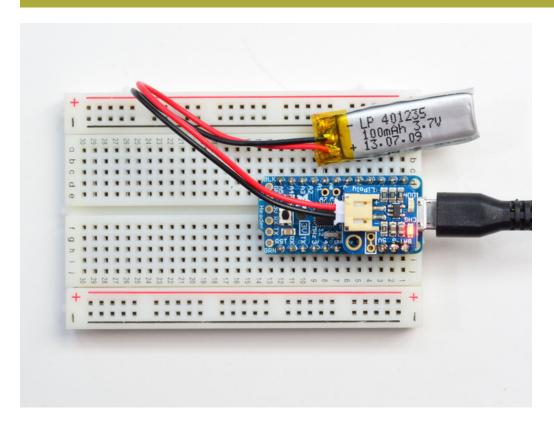
If you want to add an On/Off switch, we also made that really easy. The two 0.1" holes with a box around them are the battery output line. Carefully cut the trace between them with a hobby knife and replace with two wires from a switch like this slide switch (https://adafru.it/drN), or this pushbutton one (http://adafru.it/1683), for example.
