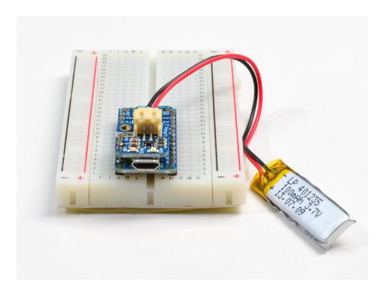
Ideally, this backpack is for use with the 3.3V Pro Trinket, so that the battery voltage (3.7V-4.2V) will get regulated down to 3.3V on the Pro Trinket board. However, many times, you can run a 5V Pro Trinket + accessories off of the "4V from the LiPoly battery with no problem. (Technically its overclocking but we've never seen that affect the Pro Trinket itself, AVRs are happy to overclock without complaint).
