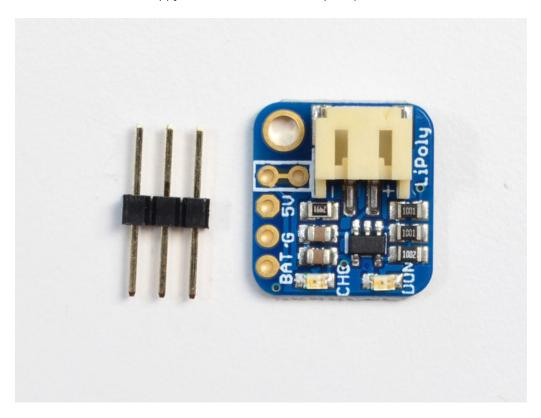
Solder the backpack on with the extra long header so that it can still plug into a breadboard, or clip the long header
