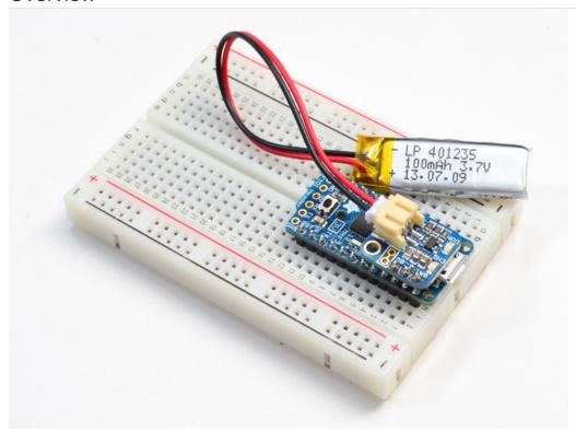
If you have a Pro Trinket you probably know it's the perfect little size for a portable project. This LiPoly backpack makes it really easy to do! Instead of wiring 2 or 3 boards together to make a charging system, this little PCB sits on top of the Pro Trinket and allows a LiPoly/Lilon battery to plug in. When the Pro Trinket USB port is powered, the battery is recharged automatically. Unplug the USB port and the Pro Trinket will switch over to the rechargeable battery.
