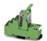
Preassembled relay modules with spring-cage connection, consisting of a relay base, industrial relay with integrated LED and engage/disengage manual actuate lever, varistor protective module, and retaining bracket. Input voltage: 230 V AC, two PDTs, 10 A
