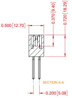
ACAD REFERENCE NO .: 317 Assembly 317 SERIES CARD EDGE CONNECTOR C.B DATE: February 5, 2020 DRAWN: CHECKED: DATE: THESE DRAWINGS AND SPECIFICATIONS OF SCALE: 1:1 SHEET 1 1 EDAC INC ARE THE PROPERTY OF EDAC INC..AND TORONTO, ONTARIO SHALL NOT BE REPRODUCED, OR COPIED 317-042-542-804 DRAWING NUMBER: ISSUE OR USED AS THE BASIS FOR THE CANADA MANUFACTURE OR SALE OF APPARATUS 1 YOUR CONNECTION TO QUALITY & SERVICE PART NUMBER: 317-042-542-804 WITHOUT WRITTEN PERMISSION.
