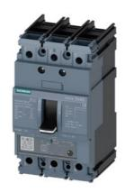
circuit breaker 3VA5 UL frame 125 breaking capacity class S 25kA @ 480 V 3-pole, line protection TM230, FTAM, In=100A overload protection Ir=100A fixed short-circuit protection Ii=5...10 x In nut keeper kit on both sides
