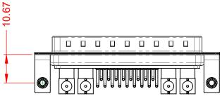
POWER/CO-AX CONTACT RATING: (IF PRESENT) SIGNAL CONTACT CURRENT RATING: 5A PER CONTACT SIGNAL CONTACT RESISTANCE:
