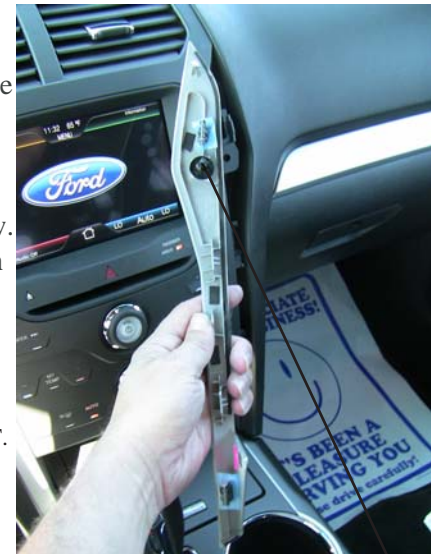
Bezel removal (plastic lug)
