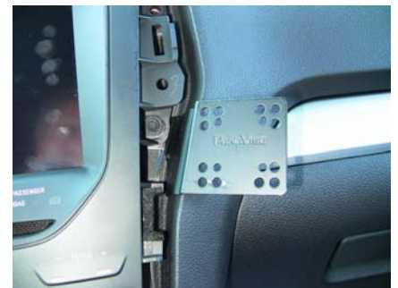
Mount installed showing screw location
