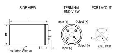
General Information Series ALN20S Dielectric Aluminum Electrolytic Description Audio Specific Aluminum Electrolytic Audio Grade Features RoHS Yes 4 Pin Solder Tags Lead AEC-Q200 No 170 g Component Weight Notes Dimensions D And L Include Sleeving.
