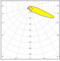
Dimensions: 35.0 mm x 35.0 mm Height: 15.35 mm Forward throwing beam with peak in 65°
