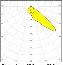
**Dimensions: 35.0 mm x 35.0 mm Height: 20.65 mm** Forward throwing beam with peak in 45°
