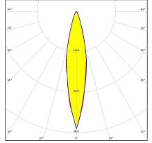
Dimensions: 35.0 mm x 35.0 mm Height: 14.52 mm ~20° beam
