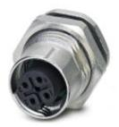
Sensor/actuator flush-type socket, 4-pos., M12 SPEEDCON, shielded, A-coded, rear/screw mounting with M12 thread, with straight solder connection
