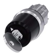
key-operated switch Siemens, 22 mm, round, metal, shiny, lock no. STGH10, with 2 keys, 2 switch positions O<I, momentary contact type, actuating angle 45°, 10:30h/12h, key removal O, with laser labeling, inscription or symbol customer-specific selection with SIRIUS ACT configurator (CIN)
