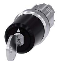
key-operated switch Siemens, 22 mm, round, metal, shiny, special lock, with 2 keys, 3 switch positions I>O<II, momentary contact type, actuating angle 2x45°, 10:30h/12h/13:30h, key removal O
