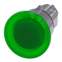
Illuminated mushroom pushbutton, 22 mm, round, metal, shiny, green, 40 mm, latching, pull-to-unlatch mechanism, with laser labeling, lower case
