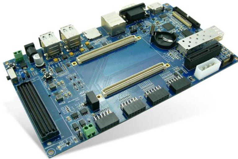
Figure 1-6 MYD-C7Z015 Base Board for MYC-C7Z015 CPU Module
