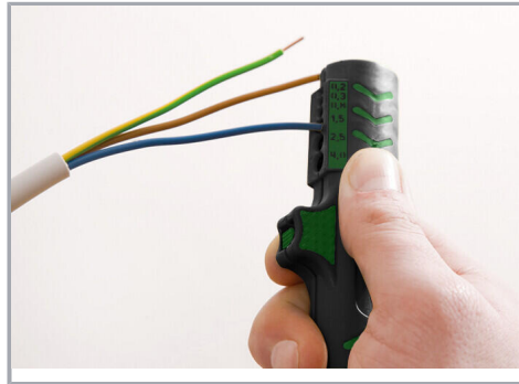
Stripping a wire insulation.
