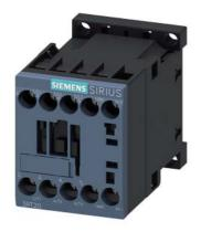
Power contactor, AC-3 16 A, 7.5 kW / 400 V 1 NO, 110 V DC 3-pole, Size S00 screw terminals
