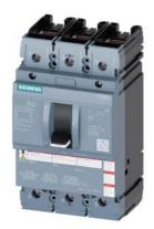
molded case switch 3VA5 UL frame 250 max. sh-circ breaking capacity 65kA @ 480 V 3-pole, line protection MCS110, ln=150A without overload protection self-protection li=16 x ln cable connection on both sides
