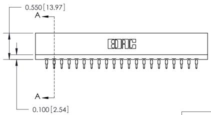
0.420 10.67 Card Slot 0.26 [6.63] 0.23 5.87 Point of Contact 0.550 13.97 0.300 [7.62] SECTION A-A
