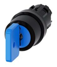
Key-operated switch O.M.R, 22 mm, round, plastic, lock number 73038, blue, with 2 keys, 3 switch positions I-O<II, left latching, right momentary contact type, actuating angle 2x45°, 10:30h/12h/13:30h, key removal O, with laser labeling, upper case and lower case,
