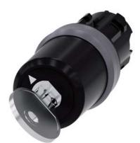
Key-operated switch BKS, 22 mm, round, plastic with metal front ring, lock number S1, with 2 keys, 2 switch positions O<I, momentary contact type, Actuating angle 45°, 10:30h/12h, key removal O, with laser labeling, upper case and lower case, always upper case at beginning of line
