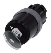
Key-operated switch BKS, 22 mm, round, plastic with metal front ring, Lock No. E7 (VW), without key, 2 switch positions O-I, latching, actuating angle  $90^{\circ}$ , 10:30h/13:30h, key removal O, with laser labeling, lower case
