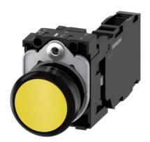
Pushbutton, 22 mm, round, plastic, yellow, pushbutton, flat, momentary contact type, with holder 1 NO+1 NC, screw terminal, with laser labeling, lower case
