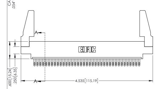
160 [4.06] POINT OF CONTACT .330[8.38] CARD SLOT **SECTION A-A**
