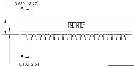
0.420 10.67 Card Slot 0.26 [6.63] 0.23 5.87 Point of Contact 0.550 13.97 0.300 [7.62] SECTION A-A
