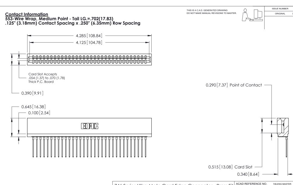
746 Series Ultra-Mate Card Edge Connector - Press Fit DRAWN: Part Number: 746-032-553-101 CHECKED: **EDAC INC** SCALE: THESE DRAWINGS AND SPECIFICATIONS ARE THE PROPERTY OF EDAC INC.,AND TORONTO, ONTARIO SHALL NOT BE REPRODUCED, OR COPIED DRAWING NUMBER CANADA OR USED AS THE BASIS FOR THE MANUFACTURE OR SALE OF APPARATUS YOUR CONNECTION TO QUALITY & SERVICE WITHOUT WRITTEN PERMISSION.
