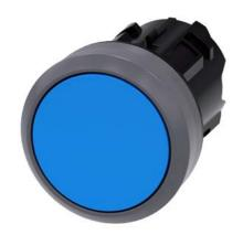
Pushbutton, 22 mm, round, plastic with metal front ring, blue, pushbutton, flat, latching, Push-to-release mechanism, with laser labeling, symbol number according to, ISO 7000 or IEC 60417
