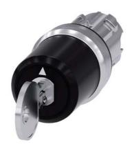
key-operated switch Siemens, 22 mm, round, metal, shiny, lock no. STGH10, with 2 keys, 3 switch positions I-O<II, left latching, momentary contact type on the right, actuating angle  $2x45^{\circ}$ , 10:30h/12h/13:30h, key removal O+I, Z=50-unit packaging
