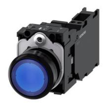
Illuminated pushbutton, 22 mm, round, plastic, blue, pushbutton, flat, momentary contact type, with holder, 1 NO+1 NC, LED module with integrated LED 24 V AC/DC, spring-type terminal, with laser labeling, upper case
