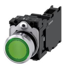
Illuminated pushbutton, 22 mm, round, Metal, shiny, green, pushbutton, flat, momentary contact type, with holder, 1 NO+1 NC, LED module with integrated LED 230 V AC, spring-type terminal, with laser labeling, upper case and lower case, always upper case at beginning of line
