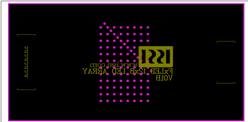
Figure 10: LED Board Component Placement Guide - Bottom Layer
