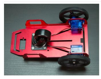
Start by screwing the DC motors to the back of the chassis (i.e. the end farther away from the angled front). Make sure the motors have the same orientation, with the side that the wire exits facing forward.
