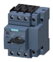
Circuit breaker size S0 for motor protection, CLASS 10 with overload relay function A-release 23...28 A N-release 364 A screw terminal Standard switching capacity
