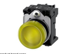
Indicator lights, 22 mm, round, metal, shiny, yellow, lens, smooth, with holder, LED module with integrated LED 230 V AC, screw terminal
