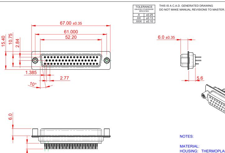
HOUSING: THERMOPLASTIC POLYESTER, UL94V-0 SHELL: STEEL, NICKEL PLATED CONTACT: COPPER ALLOY, GOLD FLASH PLATED OPERATING TEMPERATURE: -55°C to +105°C
