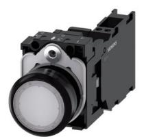
Illuminated pushbutton, 22 mm, round, plastic, white, pushbutton, flat, momentary contact type, with holder, 1 NO+1 NC, LED module with integrated LED 24 V AC/DC, spring-type terminal, with laser labeling, lower case
