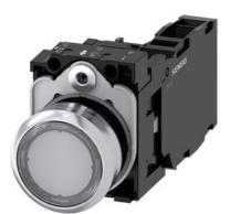
Illuminated pushbutton, 22 mm, round, metal, shiny, clear, pushbutton, flat, momentary contact type, with holder, 1 NO+1 NC, LED module with integrated LED 24 V AC/DC, screw terminal, with laser labeling, inscription or symbol Customer-specific selection with SIRIUS ACT configurator (CIN)
