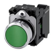
Pushbutton, 22 mm, round, metal, shiny, green, pushbutton, flat, momentary contact type, 1 NO, spring-type terminal, with laser labeling, lower case
