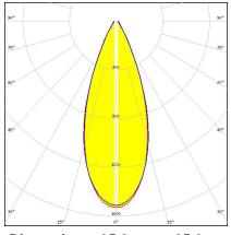
Dimensions: 35.0 mm x 35.0 mm Height: 15.00 mm ~40° wide beam with 1.5 mm high location pins
