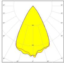
Dimensions: 35.0 mm x 35.0 mm Height: 15.00 mm ~60° wide beam with 1.5 mm high location pins. Optimized for CREE XR-E.
