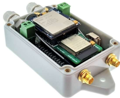
Pic. 23. LTE CAT-M1 WiFi GPS asset tracker POC
