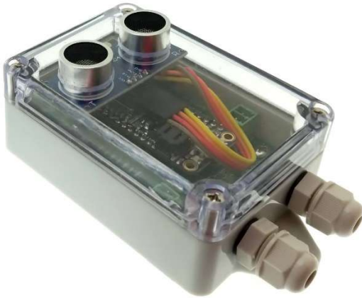
Pic. 22. WiFi Ultrasound sensor : waste collection project
