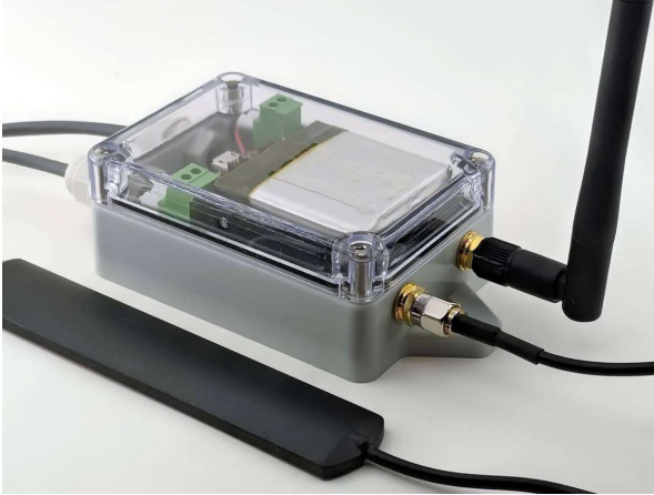
Pic. 18. LiPol battery applied to a transparent lid (assembled view)
