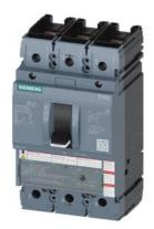
circuit breaker 3VA5 UL frame 250 breaking capacity class H 65kA @ 480 V 3-pole, line protection TM230, FTAM, In=90A overload protection Ir=90A fixed short-circuit protection Ii=5...10 x In nut keeper kit on both sides
