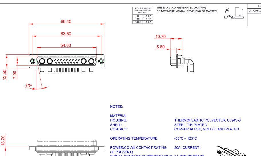
SIGNAL CONTACT CURRENT RATING: 5A PER CONTACT SIGNAL CONTACT RESISTANCE: 10mΩ MAX.
