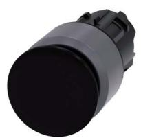
Mushroom pushbutton, 22 mm, round, plastic with metal front ring, black, 30 mm, latching, pull-to-unlatch mechanism, with laser labeling, symbol number according to, ISO 7000 or IEC 60417
