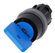
Key-operated switch O.M.R, 22 mm, round, plastic with metal front ring, lock number 73038, blue, with 2 keys, 2 switch positions O<I, momentary contact type, Actuating angle 45°, 10:30h/12h, key removal O, with laser labeling, lower case
