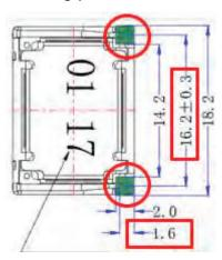
New: Pin Pitch- 16.75±.3mm Touching point- 1.5±.2mm
