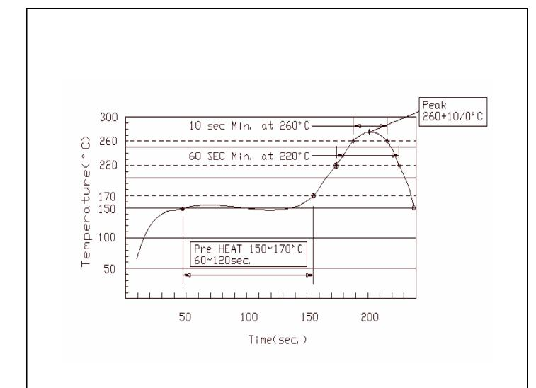
Fig. 1. Recommended Reflow Temp. Profile
